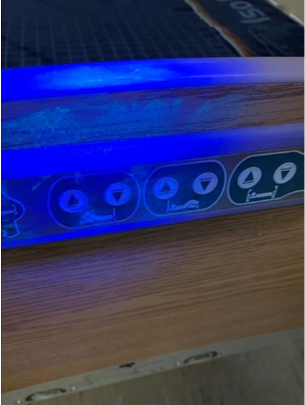
Photos showing manual disinfection (disinfection shown by the removal of the UV solution on the surface)
